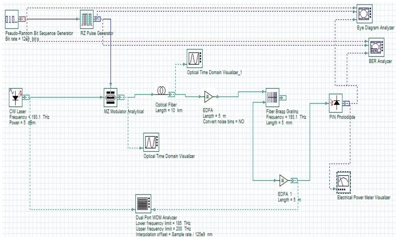
Figure 2. Simulated model of 12 GBPS optical transmission system on Opti system software
