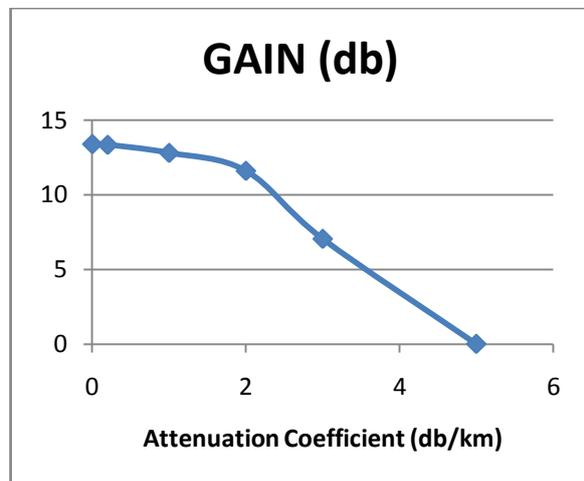
(b) Attenuation coefficient vs. Gain
