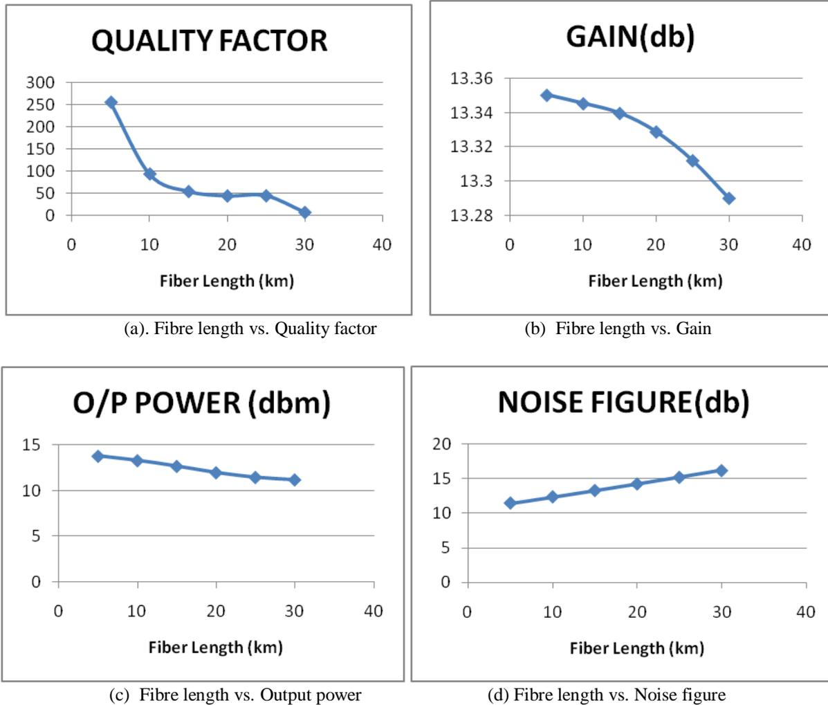
Figure 4. Graphs showing variation in (a) Quality factor, (b) Gain, (c) Output power and (d) noise figure as a function of Fiber length
