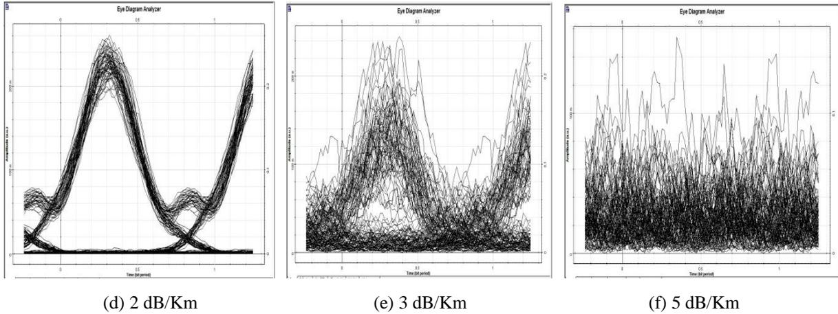
Figure 7. Eye diagram at different Attenuation coefficient.
