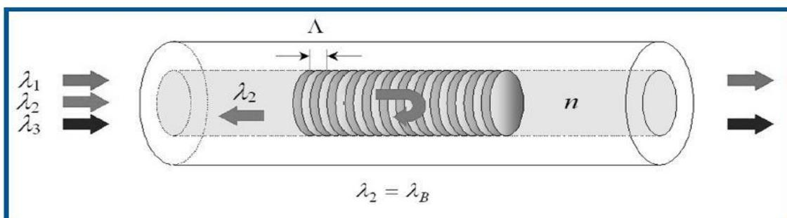
Figure 1 Principle of Fiber Bragg Grating [4]
