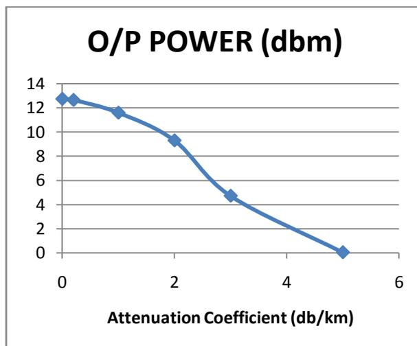
(c) Attenuation coefficient vs. Output power
