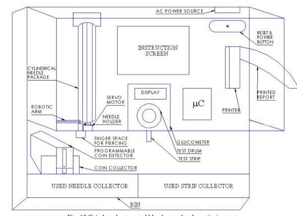
Fig. 10 Coin based automated blood sugar level monitoring system
