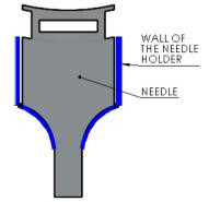
Fig. 19 Needle placed in the needle holder
