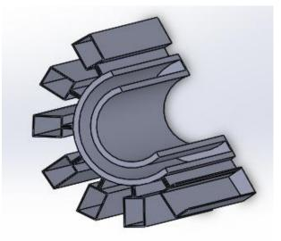
Fig 16 Cut section view of the cylindrical needle package
