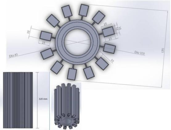
Fig. 11 Cylindrical Needle Package
