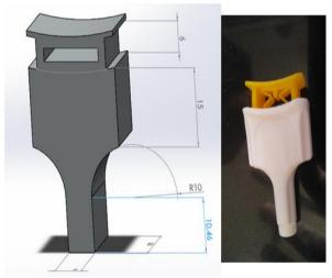
Fig. 18 Sterile needle package (before using)
