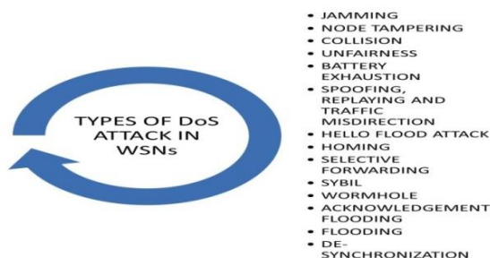
Figure 3 - Types of Denial of Attack in Wireless Sensor Network
