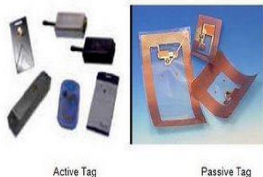
Fig 2: Active and passive tags
