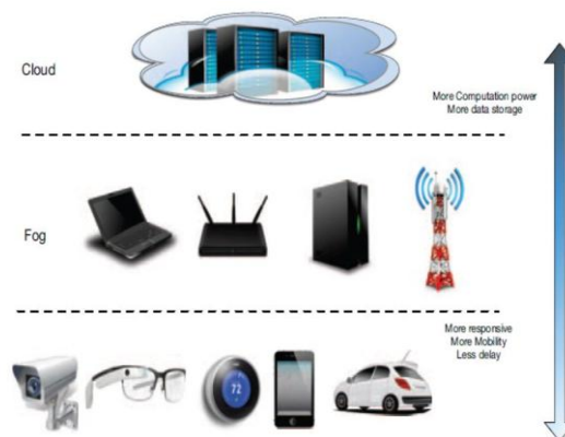
Fig. 1. Three layer architecture: end user/fog/cloud
