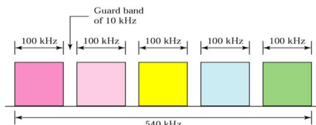
Fig. 8 Guard band in FDM
