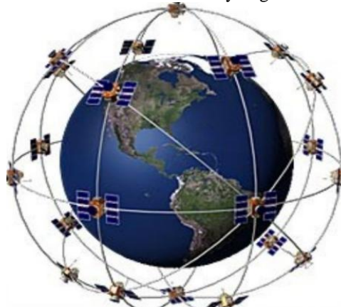
Fig. 12GPS System, 24 Satellites in 6 Orbit planes, 4 satellites in each plane, about 20200Km from earth surface
