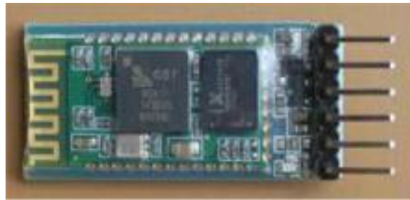
Figure 1: HC-05 Bluetooth Module
