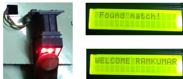
Fig.8 LCD displaying the results of Finger Print Authentication System
