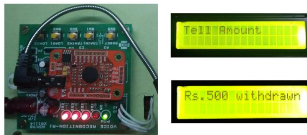
Fig.14 Voice Recognition process – LCD displaying the Amount withdraw status
