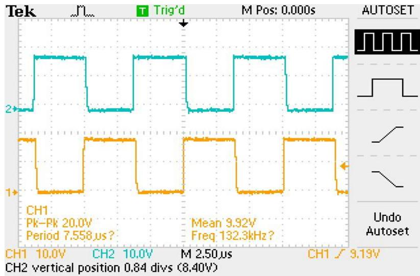
Fig. 15 : Gate pulse from driver circuit TLP250
