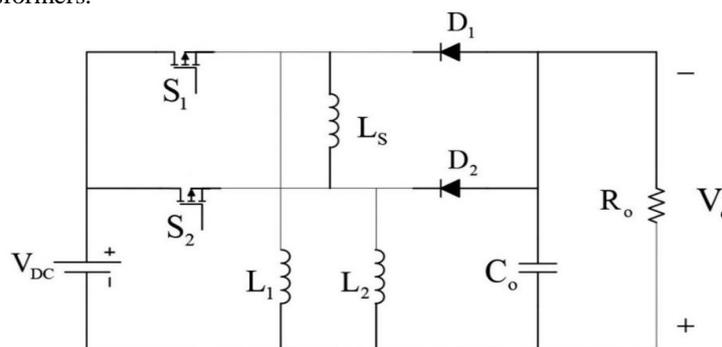
Figure 1: Configuration of parallel buck-boost converter
