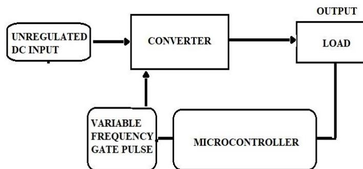
Figure 3 Schematic block diagram of closed loop voltage regulation
