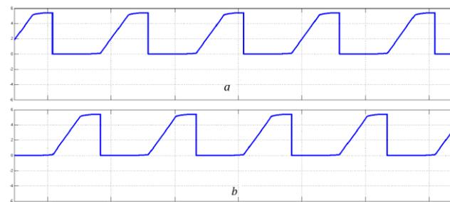
Figure 11: Simulation results of (a) current through switch S1 (b) current through switch S2
