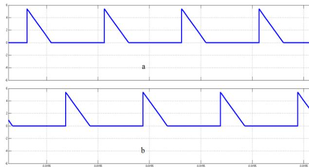
Figure 13: Simulation results of (a) current through diode D1 (b) current through diode D2
