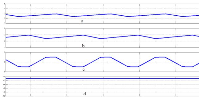
Figure 14: Simulation results of (a) current through inductor L1 (b) current through inductor L2 (c) current through inductor LS (d) voltage across output capacitor C0
