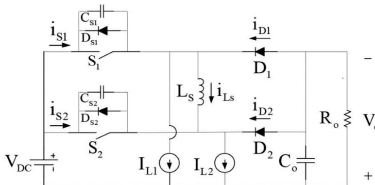
Figure 2: Equivalent circuit of the double deck converter
