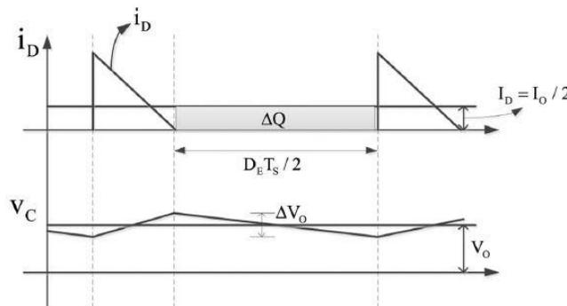
Figure 9: Diode current and output voltage ripple across the output capacitance
