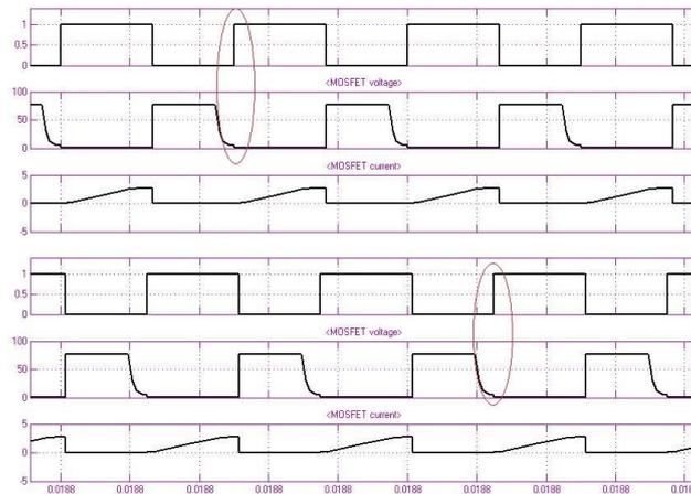
Figure 10: Simulation results of (a) Voltage across switch S1 (b) Gate pulse of switch S1 (c) Current through switch S<sub>1</sub> (d) of Voltage across switch S2 (e) Gate pulse of switch S1 (f) Current through switch S<sub>1</sub>
