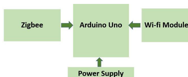
Fig.5. Block diagram of GN node
