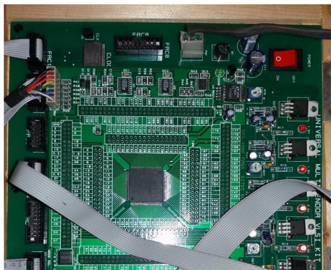
Fig.5.Hardware Implementation Output of 4 bit Vedic Multiplier
