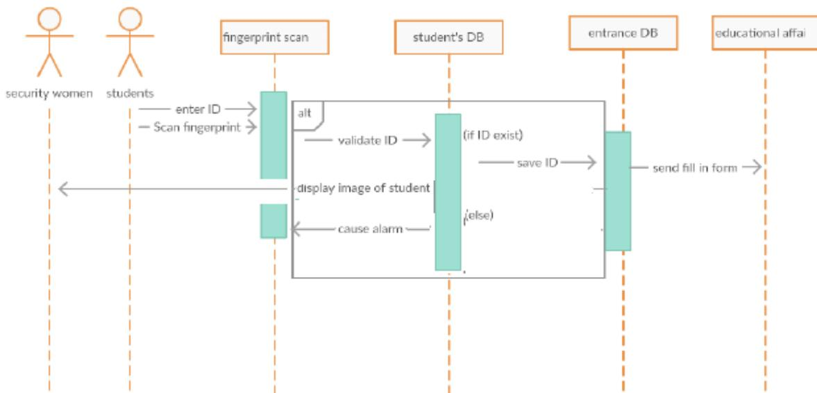
Fig. 4 Sequence diagram for the entrance using fingerprint processing
