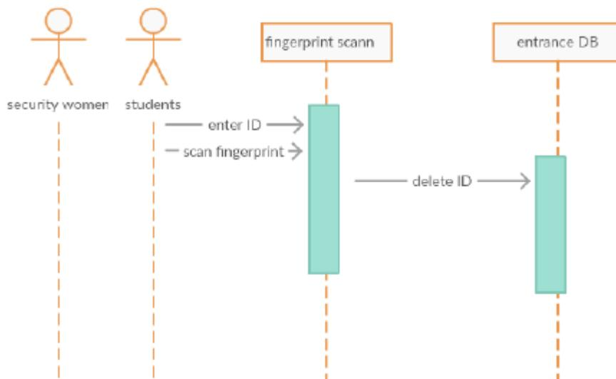
Fig. 6 Sequence diagram for the exit using fingerprint processing
