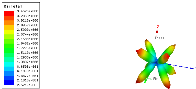
Fig. 7 3D directivity polar plot for flared antenna with arlon substrate.
