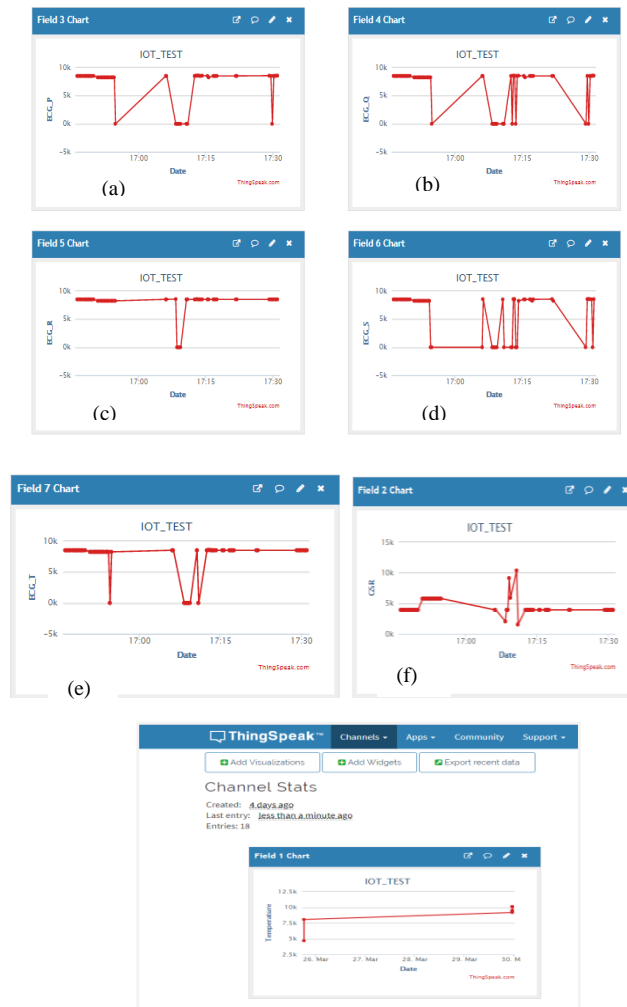
Fig. 10: (a),(b),(c),(d),(e) are PQRS encrypted value of ECG respectively. (f) is GSR and (g) is body temperature encrypted value.
