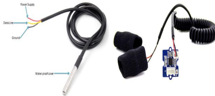
Fig. 2: DS18B20 Temperature Sensor and GSR sensor 101020052/01
