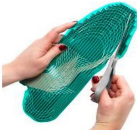
Figure 7 shows how the sensor can be cut to fit inside the shoe of a specific person
