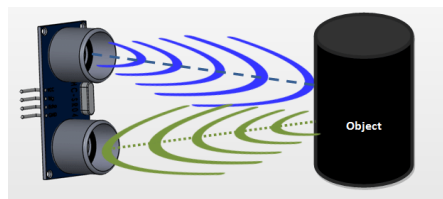
Fig.2. Ultrasonic sensor to detect human presence
