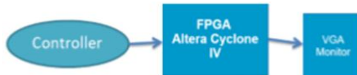
Fig. 8 Block diagram of Snake game based on FPGA
