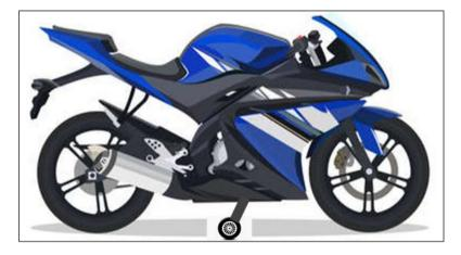
3. **Bike Skidding**: If the rider sees bad or wet roads and need to drive slowly and carefully so that the bike won't skid, the rider needs to put the switch button to Manual mode. In this situation, the balancing wheels will be deflated which will balance the bike. Possibility of bike skidding due to bad roads or wet roads. To avoid skidding, this system will balance the bike and let the driver focus on acceleration and brakes.
