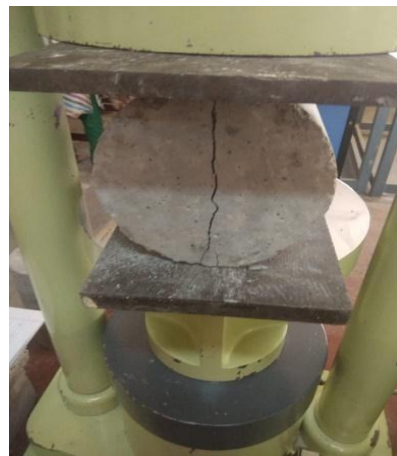
Fig. 12 Split Tensile Strength Test
