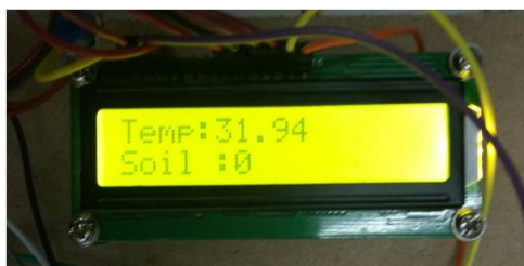
Figure 3: Soil Moisture sensor On the LCD
