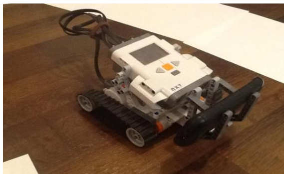
Figure 2: An Image of the Lego robot as it is driving along its course, close up look at the holder mechanism for the Android phone.
