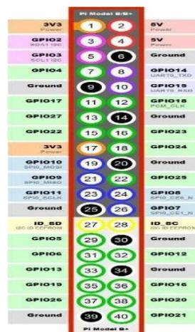
Fig. 2 Pin Diagram Raspberry Pi
