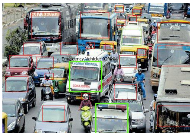
Fig. 6. Recognition of vehicles in OpenCV
