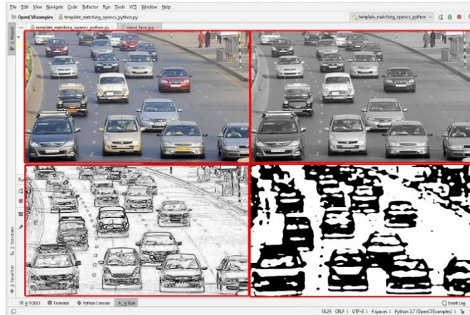
Fig. 5. Processing of digital image by OpenCV
