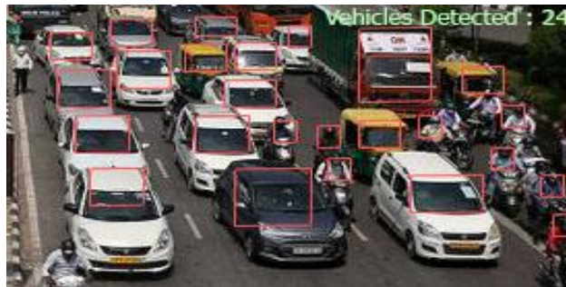
Fig. 7. Extraction of data (Vehicle count) in OpenCV
