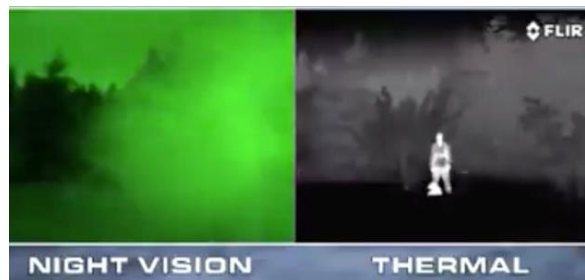
Figure 2. Representative image showing the same frame taken with night vision and thermal camera. Source FLIR.
