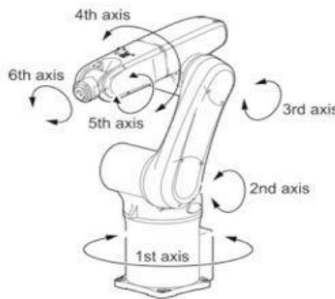
Fig. 1 Basic Mechanism of a Robotic Arm
