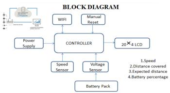
The rpm of front wheel is used for calculating the speed. The standard relation of speed, distance and time is used to calculate the distance covered by the electric bike.
