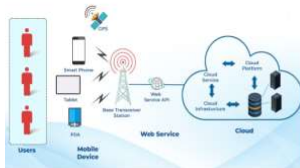
Fig 3. Mobile cloud computing system architecture(Source:ESDS-Exploring Mobile Cloud Computing)
