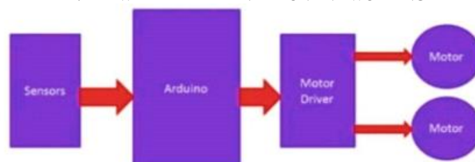
Fig. 1 Block diagram of Line following Robot
