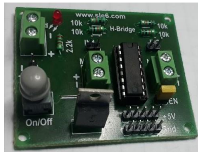
Fig : L293D Integrated Chip(IC) has driver circuit.
