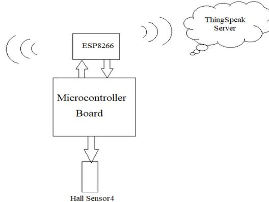
When theft is detected at the client side then microcontroller communicates with IOT. Then by using Wi-Fi microchip and IOT (thing Speak Server) platform it notify electricity board about power theft.
