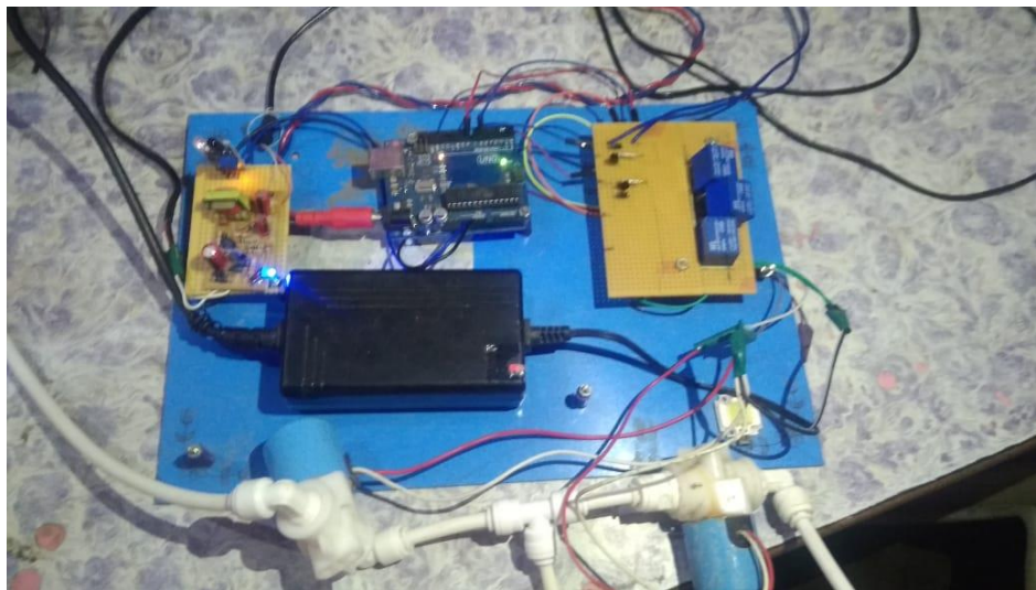
Fig. 8 Dynamic Faucet using Arduino
