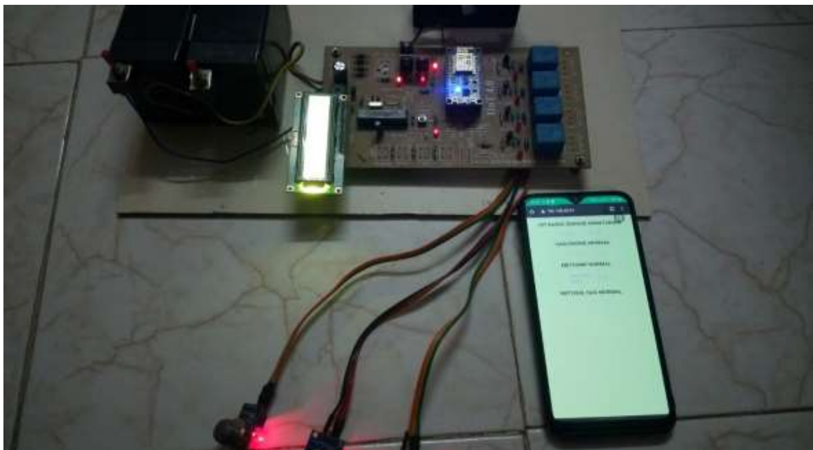
Fig.2 Pollution Monitoring and Controlling Output
