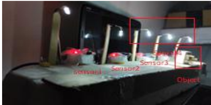
(Fig. 5.2: Last three LED glow at more intensity when object found near sensor4 during night)
