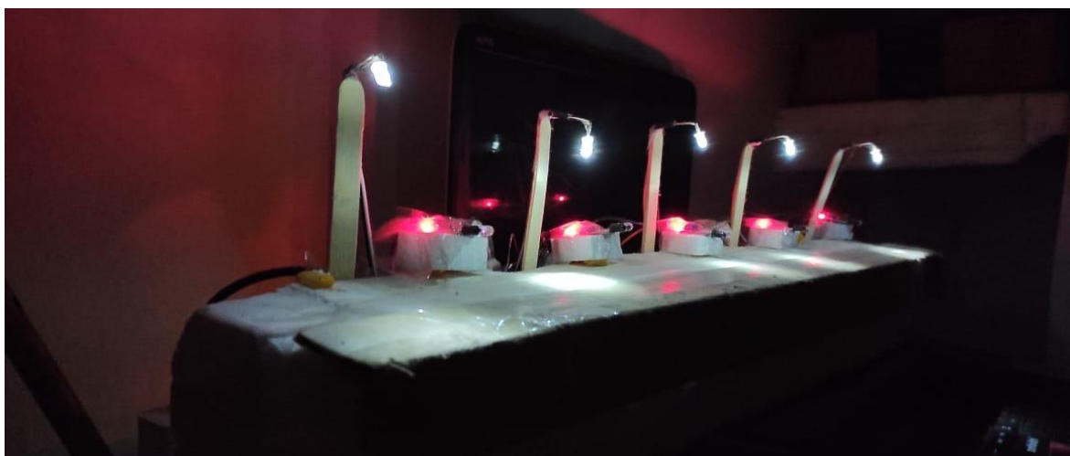
(Fig. 5.1: LED are dim when no object found near them during night)
