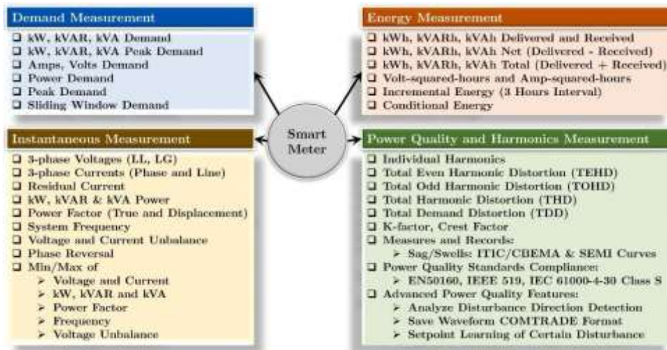
Fig. 2. Measurement and monitoring capabilities of smart meter
