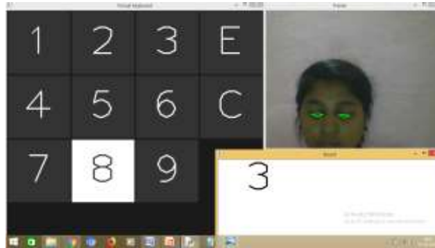
Figure 6.4 Virtual keypad taking input through eyes.
