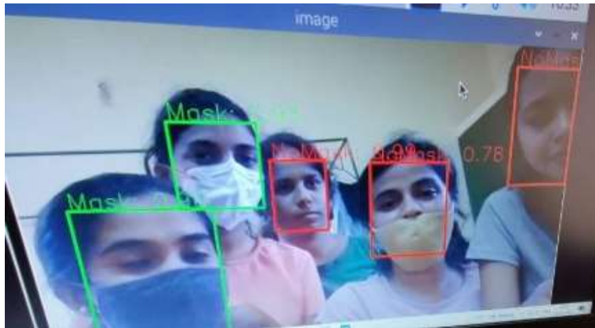
Figure: Video Stream Display of a Person Wearing a Mask or Not
