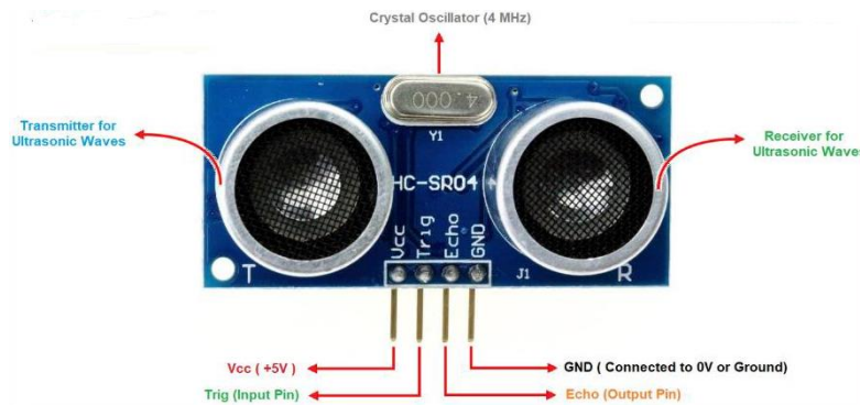
Fig. 3 HC-SR04 distance sensor
