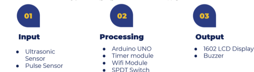
Fig. 1. Technical implementation of “Be Fit Smart Band”
