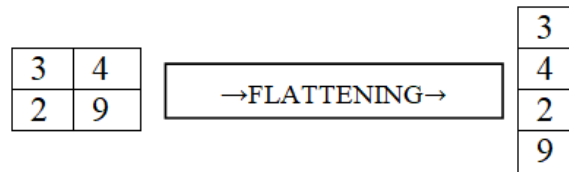
Figure 4: Working of a Flattening layer
