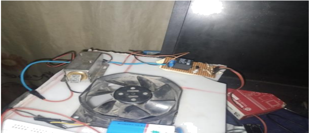
Figure 4 Output Unit: Solenoid Lock and buzzer.
