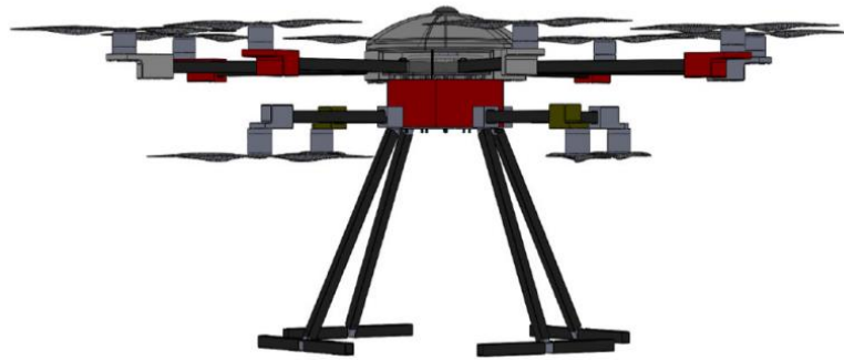
Fig. 2. Solid model of the universal drone system.
