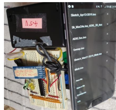
Fig. 9 Programming of a microcontroller by Android Smartphone.
