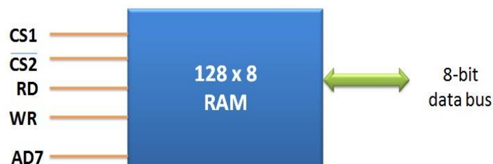
Block Diagram Representing 128 x 8 RAM (Random Access Memory)
