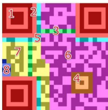
Figure 4. Structure of QR Code
