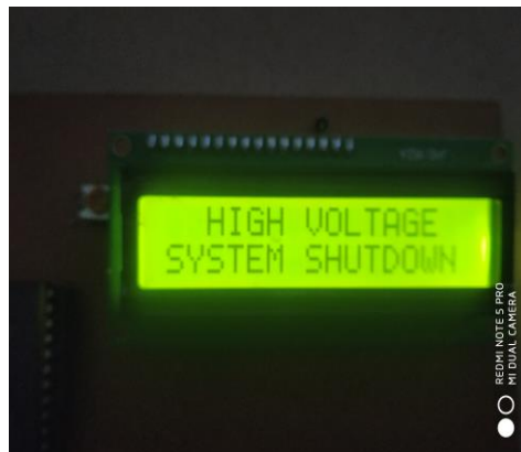
Fig. Fig. 2(c) High Voltage indication (System shutdown) on LCD Display
