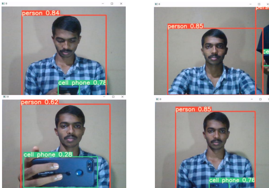
Fig. 6 Mobile and additional person detection using yolov5.
