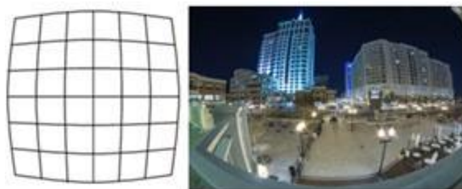
Fig. 4. Example of a distorted pattern along with a picture taken with wide- angle lens. Though able to fit in more of the physical scenery as compared to Fig. 3, the picture suffers from significant optical (barrel) distortion that can affect the representations of objects present within the image. Source: Google images.
