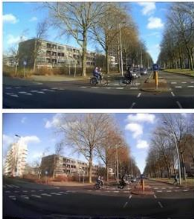
Fig. 1. Cameras with a wider field-of-view (bottom) are able to capture more imagery within the same physical space as opposed to those with a smaller field-of-view (top). Source: Google images.
