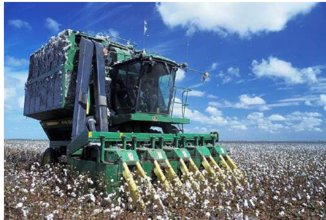
Fig. 6 Mechanised agriculture: from the first models in the 1940s, tools like a cotton picker could replace 50 farmworkers, at the price of increased use of fossil fuel.
