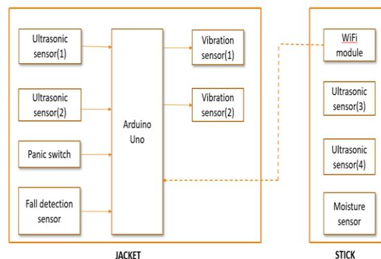
1. Arduino Uno is located at the center of the block diagram forms the control unit of the entire project.
